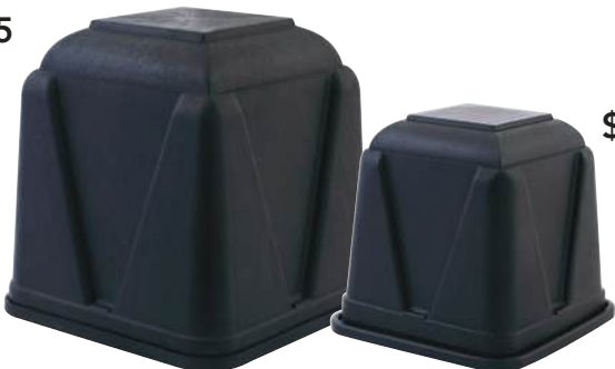
VANTAGE® 71010463 BLACK VAULT LARGE Outside Dimensions: 18.625" H x 18.5" W x 18.5" D Inside Dimensions: 15.75" H x 15.375" W x 15.375" D load tested up to 5,000 lbs per square foot
